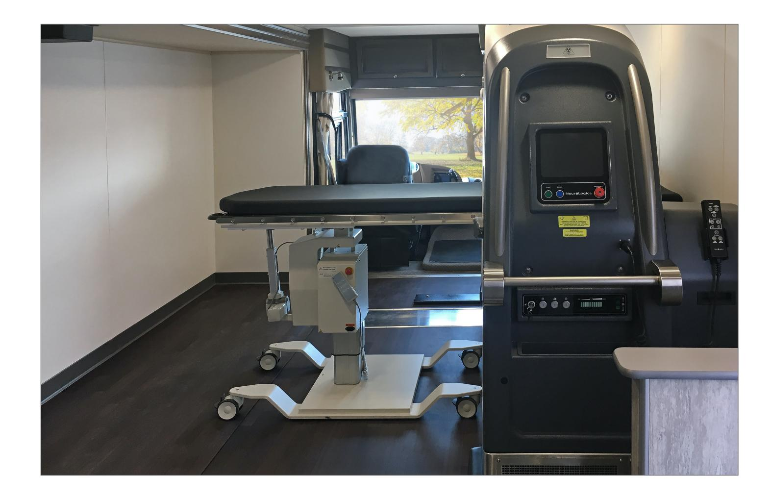
**Approach:** The Mobile CT Clinic features the BodyTom Elite, the world's first portable battery-powered full-body 32-slice CT scanner. A lithium-ion battery-based energy management system replaces the traditional generator to provide on-board power while reducing vehicle emissions.
